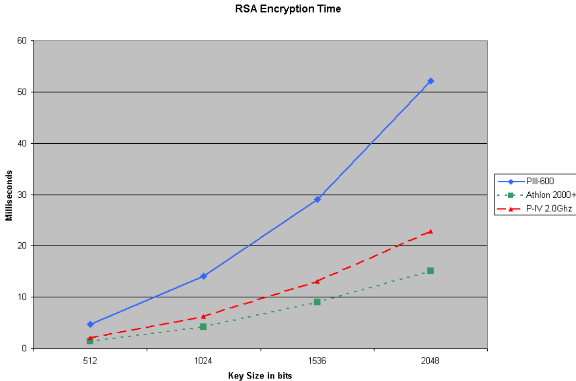
Figure 5.5: Here we plotted the encryption time in milliseconds for different RSA key lengths listed in bits. There is a line graph for each of the three test platforms: Pentium III 600MHz, Athlon XP 2000+, and P-IV 2.0GHz. Each test ran three times with 100 iterations per test.
